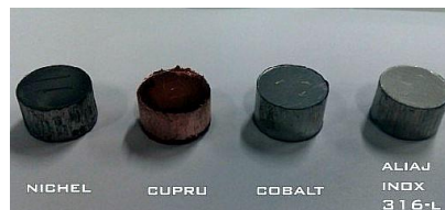
Figure 23. The metallic samples are ready to be sintered.
